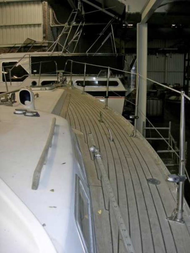
Fig. 1 Starboard side, with chainplates, stanchion bases, genoa track, handrails, and water fill caps
