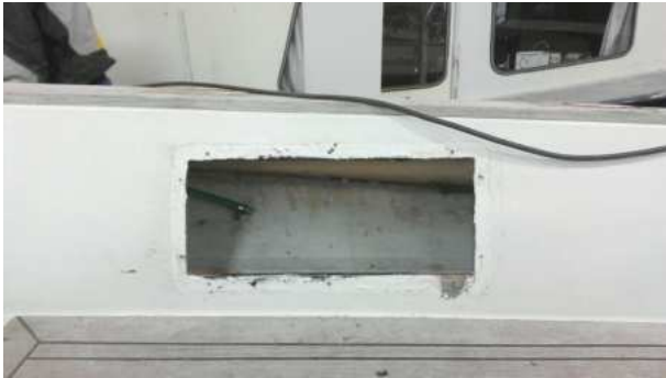
Fig. 3 The hole from the starboard storage compartment
