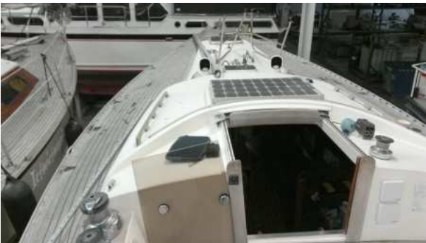
Fig. 2 Port side, stanchion bases and chainplates removed, genoa track still in place
