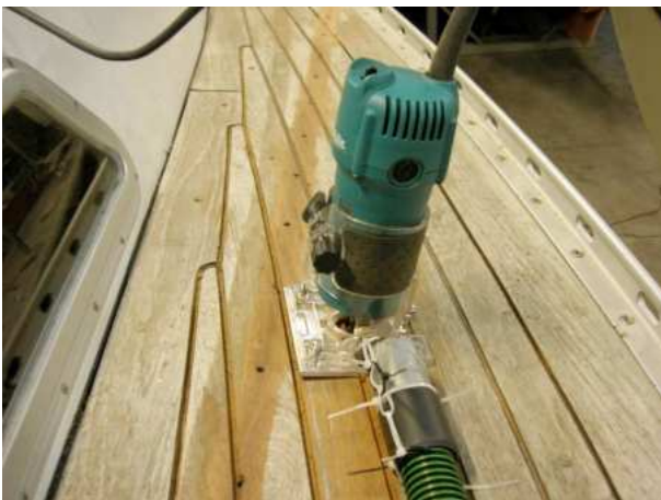
Fig. 11 Router with vacuum cleaner hose, for material extraction
