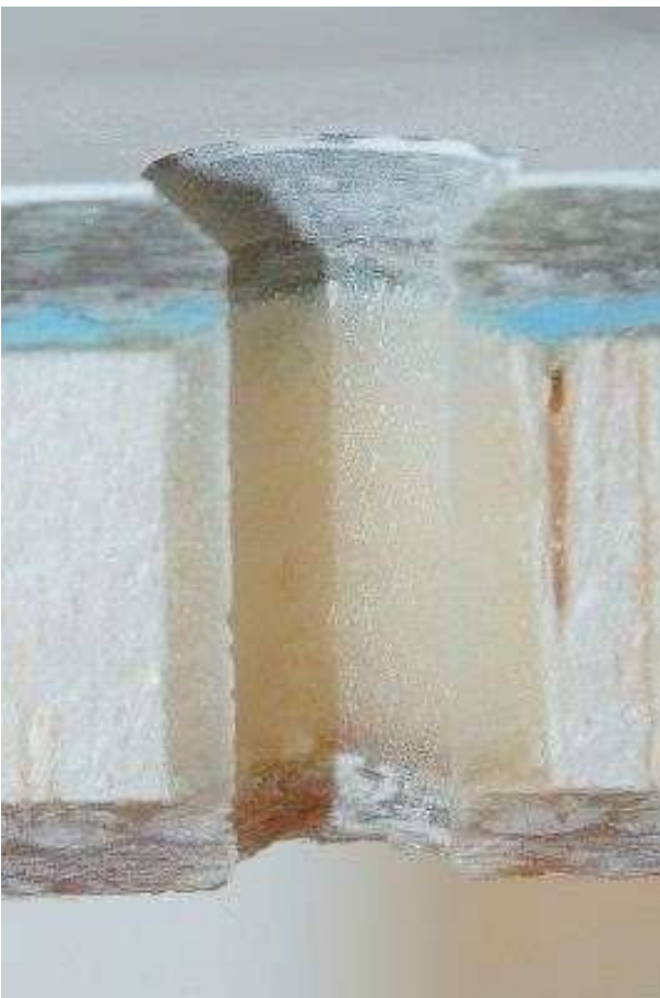
Fig. 6. A potted hole and newly drilled
