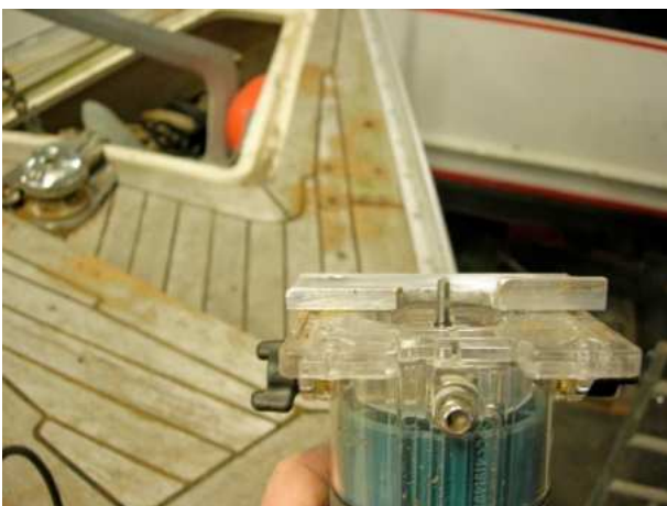
Fig. 9 Router (upside down) with router bit and attached guide
