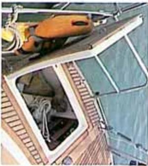
**Sail and anchor locker.** The large sail locker in the forepeak can be reached by way of a hatch in the foredeck. Here is space for ropes and other items. The anchor, with 50 metre x 10 mm (over 160ft.) anchor chain is stored here also, in its own locker.
